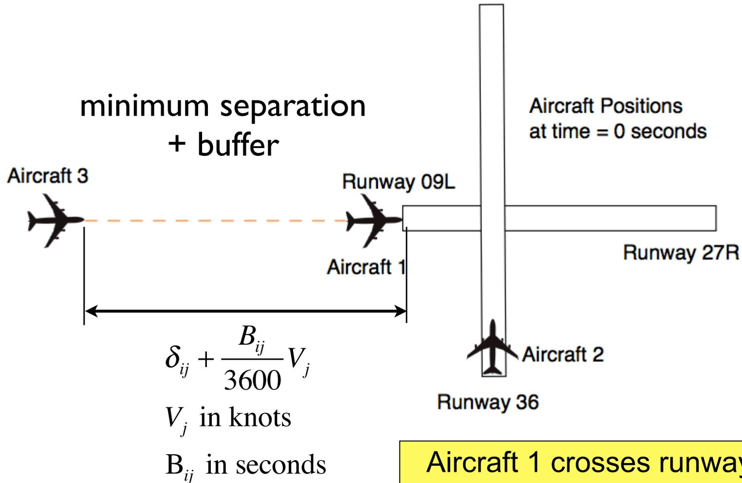
Aircraft 1 crosses runway 09L threshold . Aircraft 3 follows in-trail at the required separation behind aircraft 1
