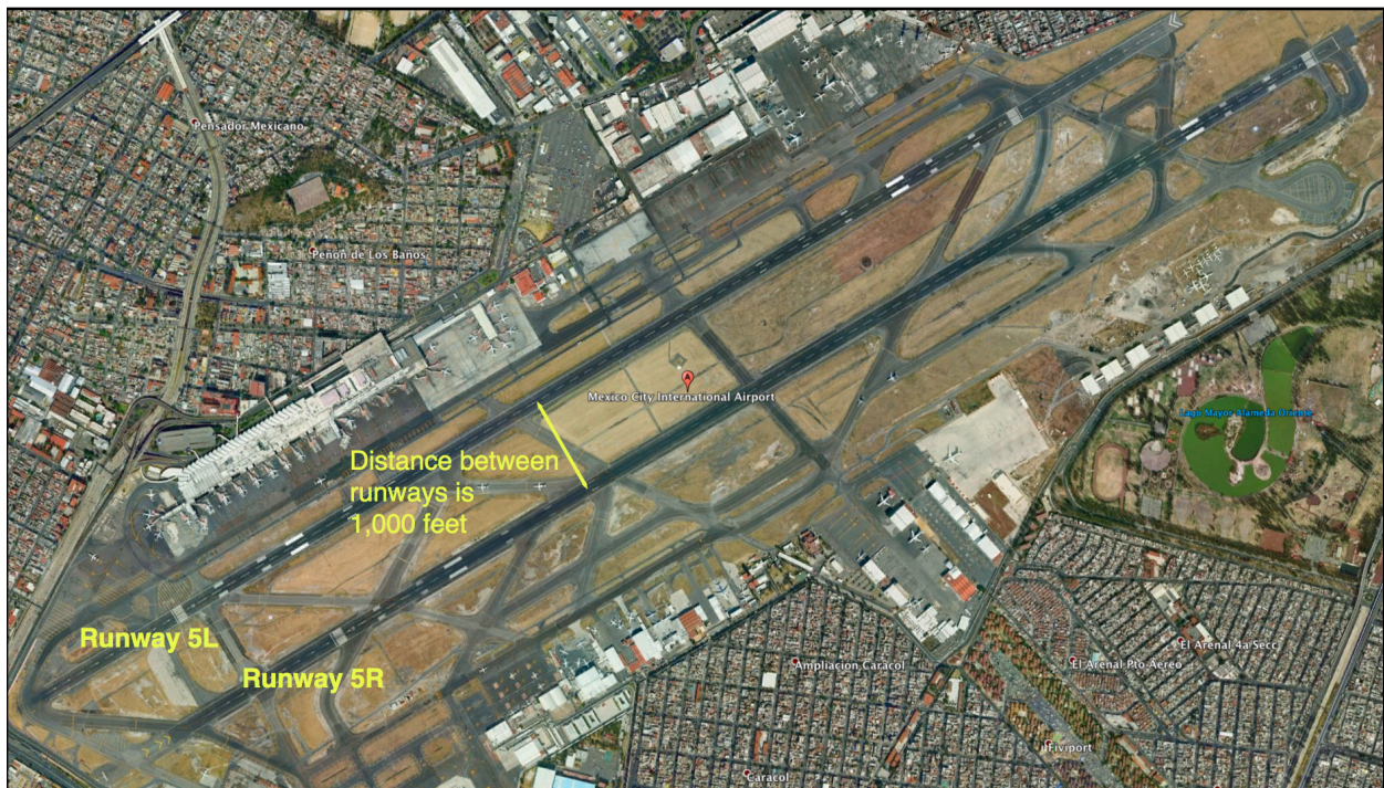
Figure 2. Mexico City International Airport Layout. Source: Google Earth 2013. Runways 5R and 5L are separated 1,000 feet. Runway 5R is used for arrivals and 5L for departures.
